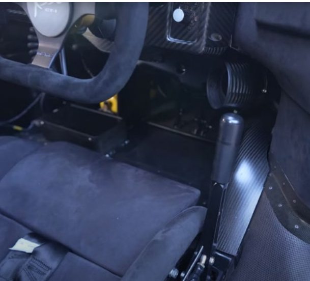
Cooling air tube goes below the dashboard
